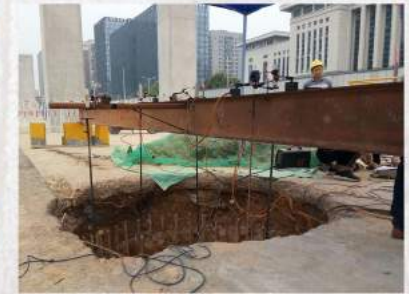
Set up the reference beam
